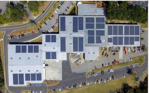
The 918kW DC standing seam, roof mounted solar PV system was installed by Hannah Solar Government Services for Hubner Manufacturing Corporation, located in Mount Pleasant, SC. This system features Canadian Solar modules connected to SMA Sunny Tripower inverters and supported by a UNIRAC mounting system. This is Mount Pleasant's largest roof mounted solar PV systems, and the largest roof mounted solar energy system in SCE&G's Distributed Energy Resource Program.
